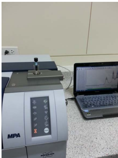
Figure 1. Near infrared scanning of orange juice sample using FT-NIR spectrometer.
