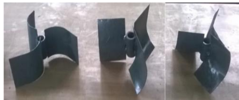
Figure 6. Various Profile of runner used for the power production.
